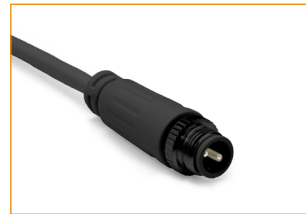
AD007-2-MCB Male connector, 30cm (0.98ft) black cable, 2 pin, IP67, Wet, 18 AWG
