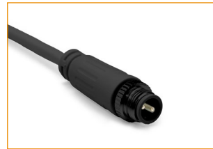
AD102-2-MCW Male connector, 30cm (0.98ft) black cable, 2 pin, IP67, Wet, 20 AWG
