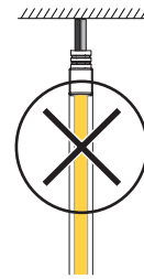
Do not suspend the power cable
