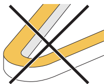
Bend too tight
