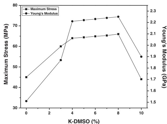
Fig. 7. Variation of max. stress and modulus Vs kaolinite content in the nanocomposites.
