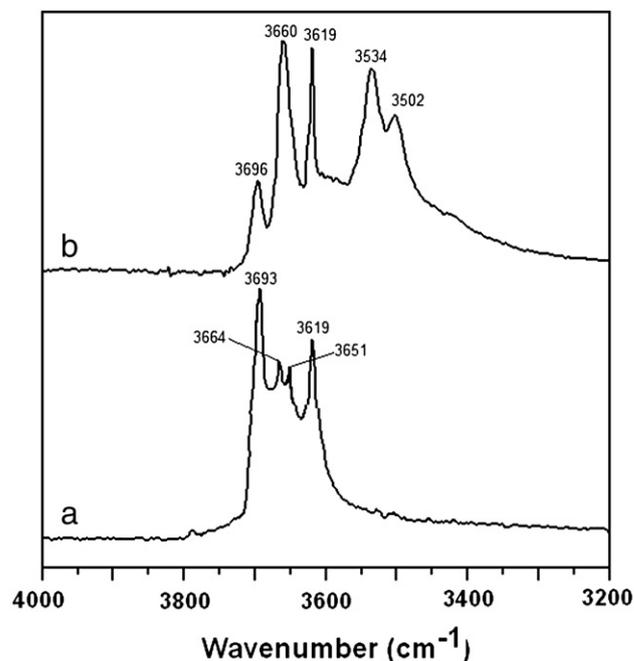
Fig. 2. FTIR spectra of (a) pure kaolinite and (b) K-DMSO.
