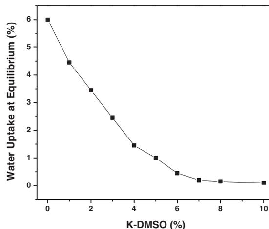
Fig. 10. Water uptake of copolymer/K-DMSO nanocomposites.
