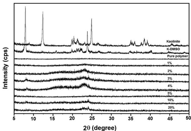
Fig. 4. XRD patterns of kaolinite, K-DMSO, pure copolymer and its nanocomposites.
