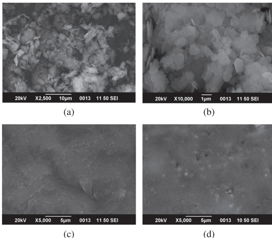
Fig. 6. SEM micrographs of (a & b) kaolinite, (c) 1-wt.% and (d) 5-wt.% of K-DMSO in the nanocomposites.
