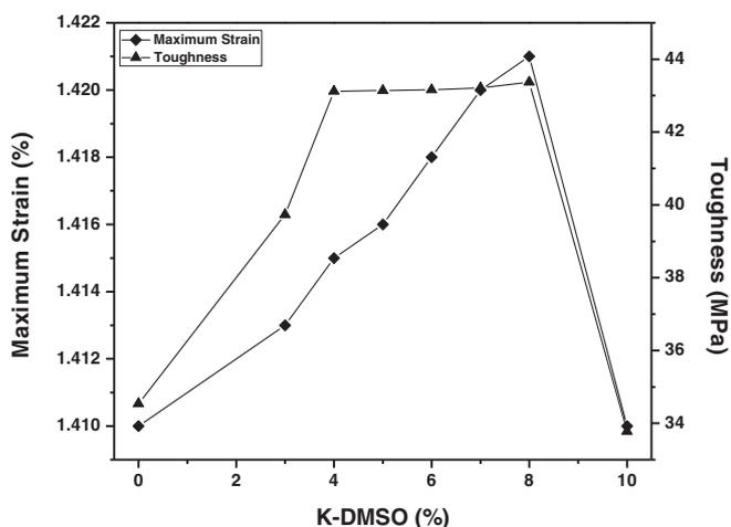
Fig. 8. Variation of strain and toughness Vs kaolinite content in the nanocomposites.
