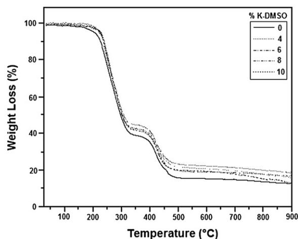
Fig. 9. TGA curves of (0) pure copolymer, 4, 6, 8 & 10-wt.% K-DMSO in nanocomposites.
