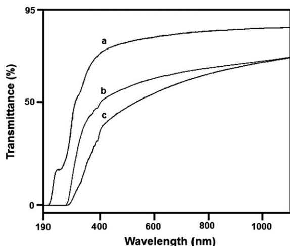
Fig. 1. UV–vis transmittance spectra of (a) pure copolymer, (b) 3-wt.%, and (c) 4-wt.% of K-DMSO in the nanocomposites.
