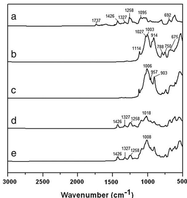
Fig. 3. FTIR spectra of (a) pure copolymer, (b) kaolinite, (c) K-DMSO, (d) 3-wt.% & (e) 4-wt.% K-DMSO in the nanocomposites.
