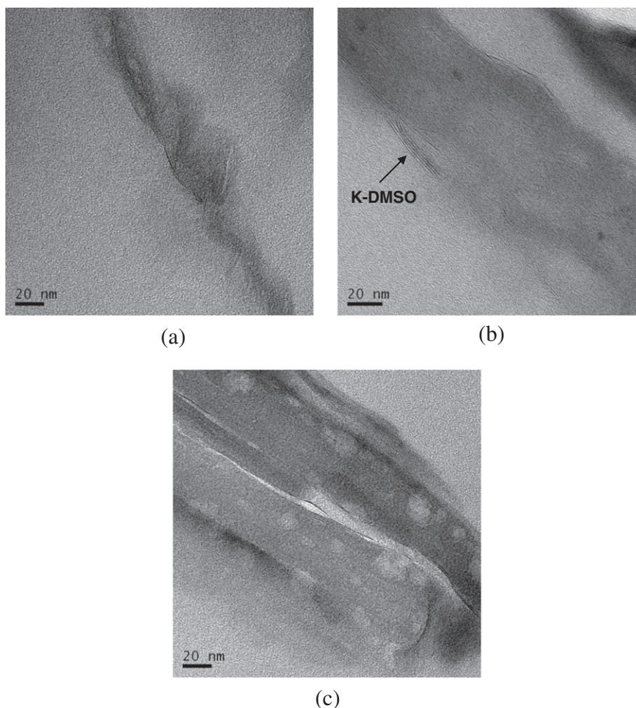
Fig. 5. TEM micrographs of copolymer/K-DMSO nanocomposites: (a) 1-wt.%, (b) 5-wt.%, and (c) 10-wt.%.
