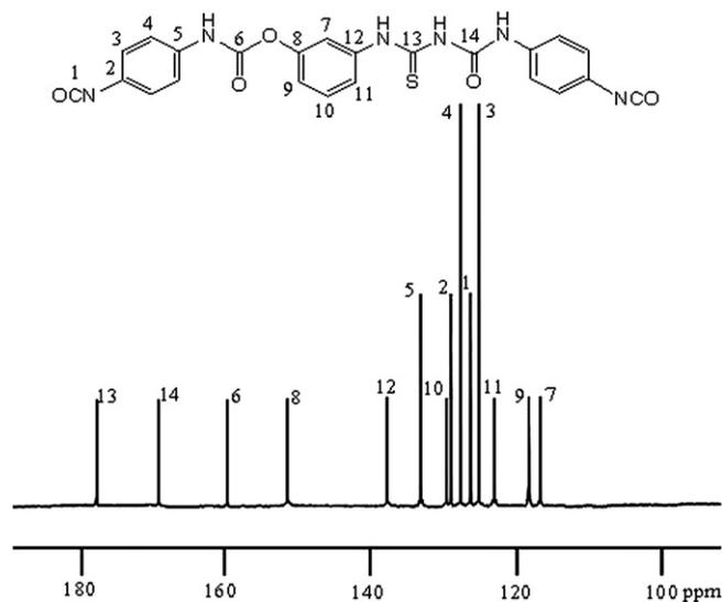
Fig. 3.  $^{13}\text{C}$  NMR spectrum of IPCT.
