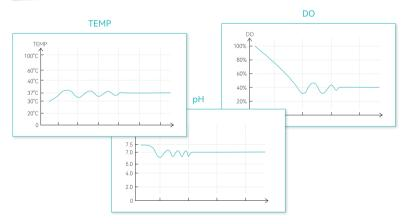
Precise PID control strategy ensures gentle fluctuations in temperature, pH, and DO, bringing the culture environment closer to a steady state.
